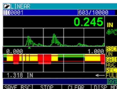
MXG 9DLW – Includes Waveform, Datalogger, B-scan, Coating Thickness, Temperature Correction, Rubber Boot
