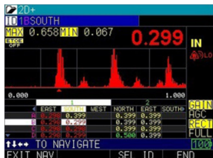
MXG 9DL – Includes Datalogger, B-scan, Temperature Correction. Gridview A-scan shown above.
